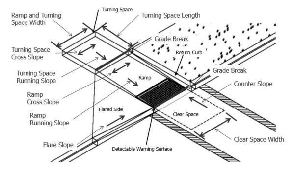
Turning Space must be level with both running and cross slopes < 2%, meaning these slopes should be designed at < 1.5% to ensure a compliant result.
