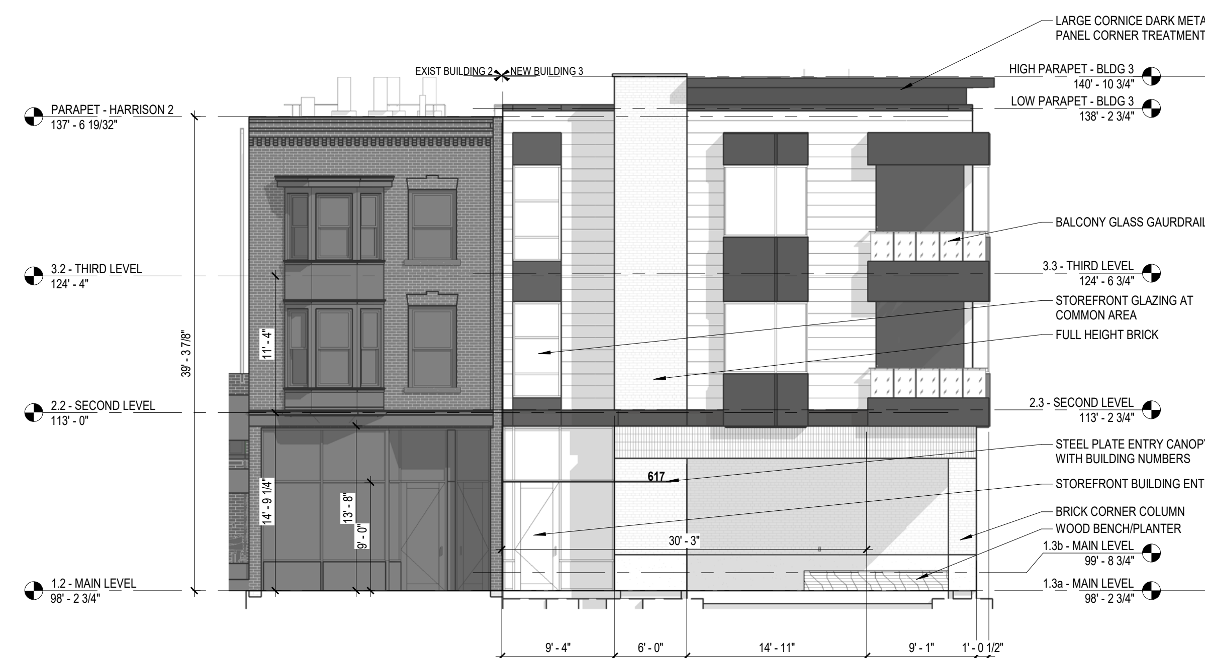
3 EXTERIOR ELEVATION - WEST - NEW BUILDING 3 SCALE: 1/8" = 1'-0"
