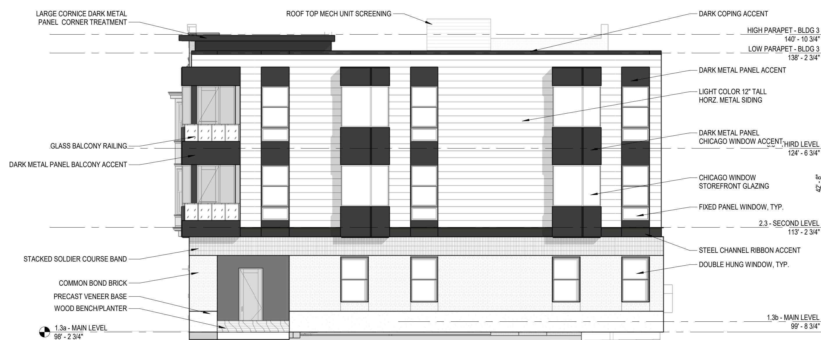
1 EXTERIOR ELEVATION - SOUTH - NEW BUILDING 3 SCALE: 1/8" = 1'-0"
