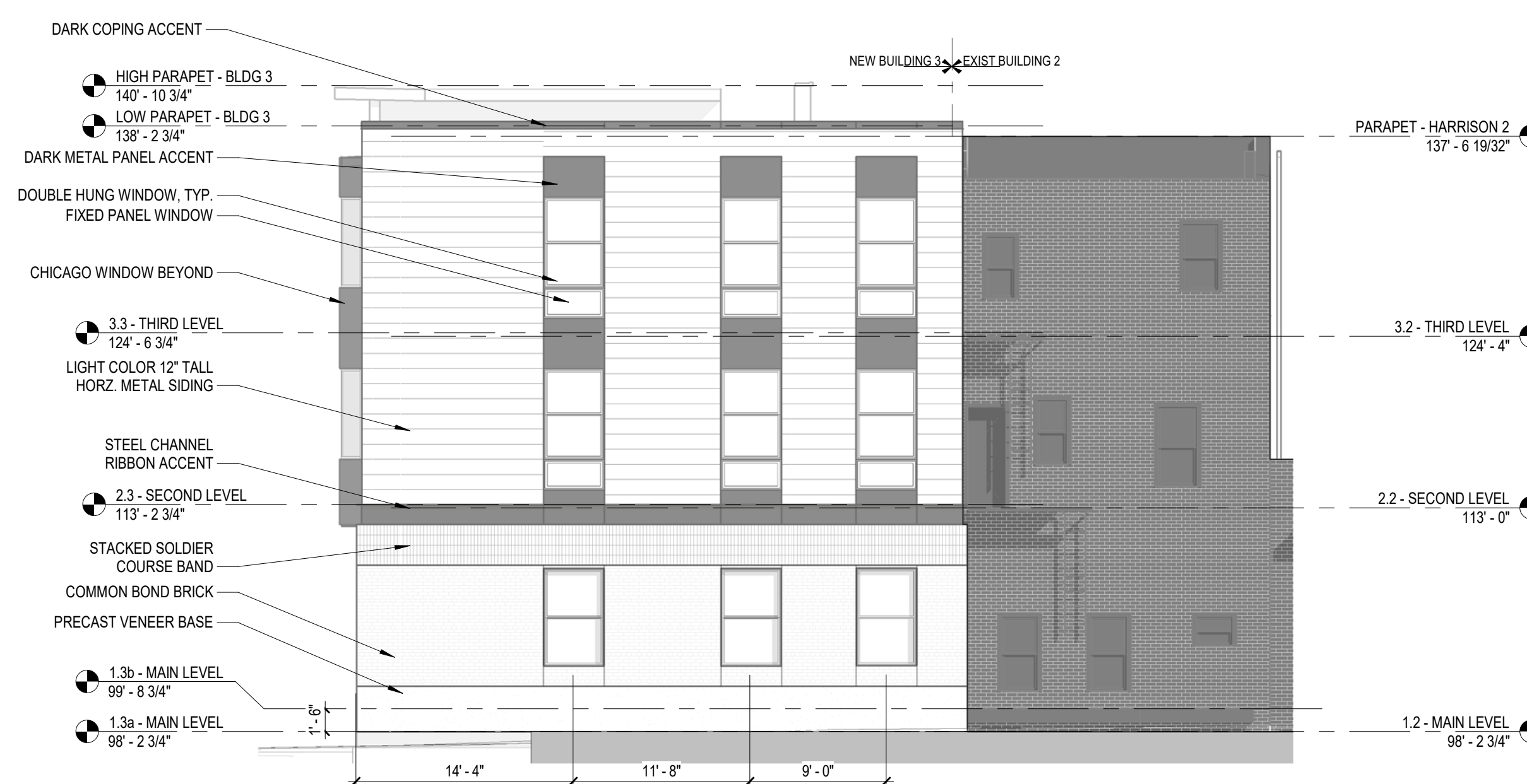
2 EXTERIOR ELEVATION - EAST - NEW BUILDING 3 SCALE: 1/8" = 1'-0"
